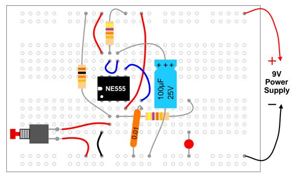
Monostable Circuit on Breadboard
