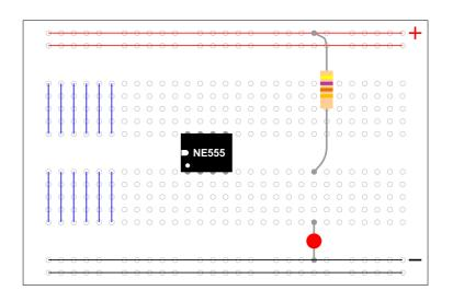
The top and bottom rows are linked **horizontally** all the way across. The power supply is connected to these rows, + at the top and 0V (zero volts) at the bottom. I suggest using the upper row of the bottom pair for 0V, then you can use the lower row for the negative supply with circuits requiring a dual supply (e.g. +9V, 0V, -9V).
